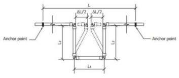
Response – The S-4 calculator makes it easy to select materials and enter required values. For a 100 foot length of PEX, we find that we will have an expansion length  $\Delta L$  of 5.5 in. The loop dimensions required to take this length change is 8.4 in X
