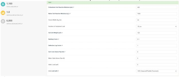
After entering these values, we can see what the critical buckling pressure is and what the resultant total load is for this installation. We are given an allowed 6,800 psi with an applied load of 1,160 psi. The final burial results in a vertical deflection of 1.8% which is well within specification.
